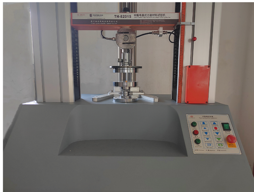
Figure 8. Compression test by a universal testing machine.
