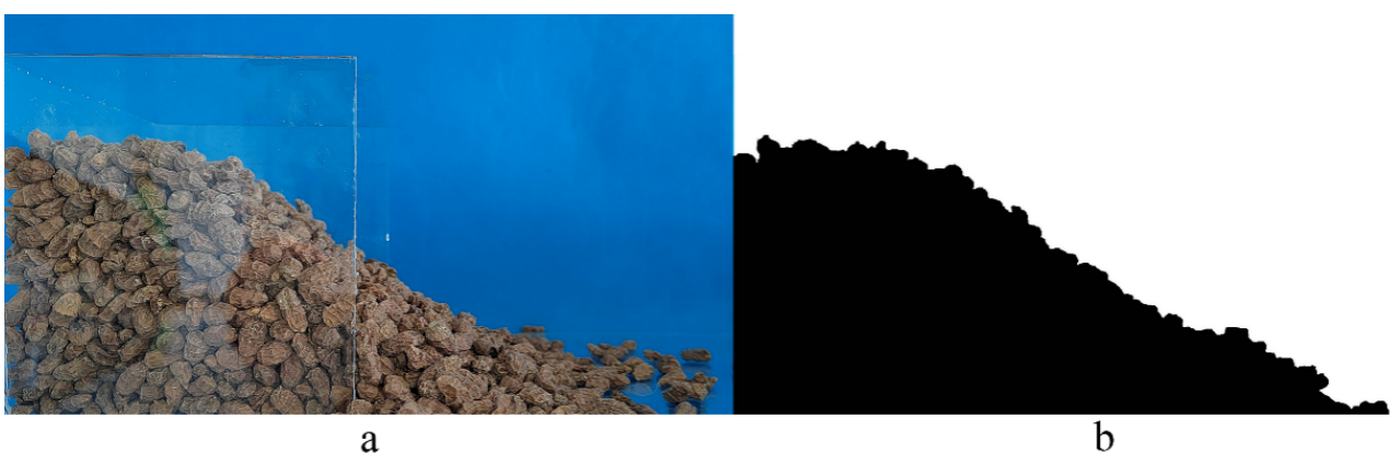
Figure 19. Packing test: (a) photograph of the piling test captured by a high-speed camera; (b) image binarization.
