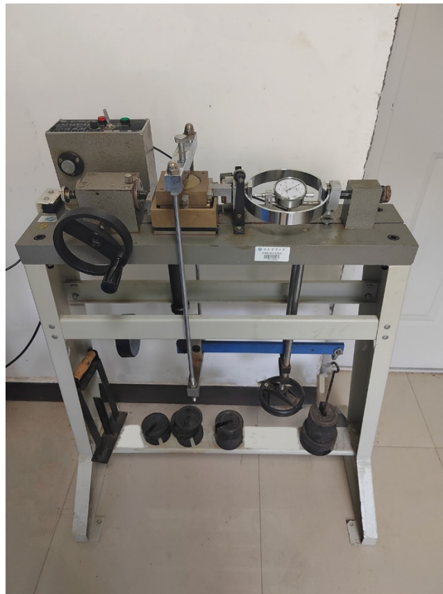
Figure 16. ZJ strain-controlled direct shear apparatus.
