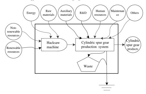
Figure 1. Emergy flow of gear manufacturing.
