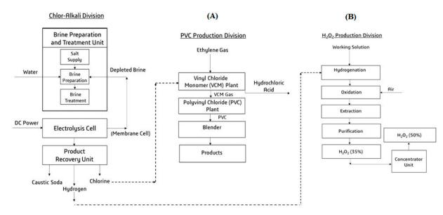
**Figure 7.** Combined Process Flow Diagram of Chlor-Alkali Process and PVC Processing Using Chlorine (**A**) and Integration of Chlor-Alkali Process and H<sub>2</sub>O<sub>2</sub> production Unit (**B**).
