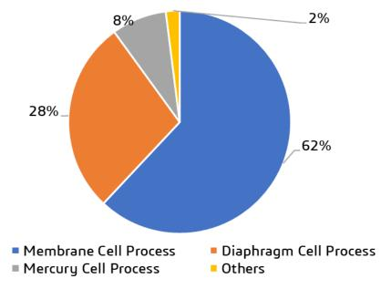
**Figure 3.** The division of capacity among the three principal cell technologies used in the world for chlor-alkali process [5].
