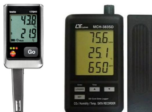
Figure 5. Recording instruments for temperature and RH (Testo 175H1) and CO 2 (MCH-383SD).
