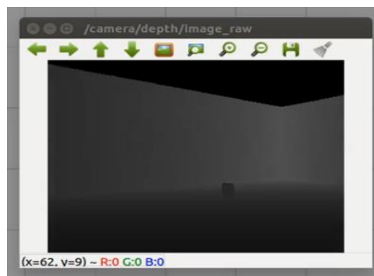
Figure 11. The depth image of the target object from an RGB–D camera.
