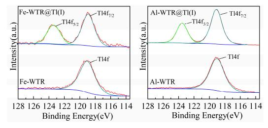
Figure 10. Tl 4f spectra of Al-WTR and Fe-WTR before and after adsorption.
