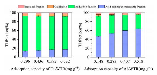
**Figure 7.** Occurrence forms of Tl(I) elements adsorbed by Fe-WTR and Al-WTR under different adsorption.
