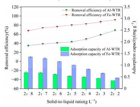
Figure 6. Effects of different solid–liquid ratios on adsorption of Tl(I) by Fe-WTR and Al-WTR.
