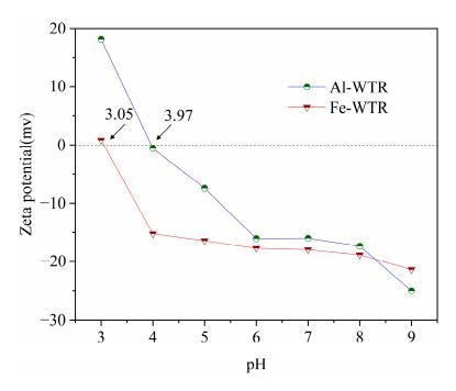
Figure 4. Zeta potential diagram of Fe-WTR and Al-WTR.
