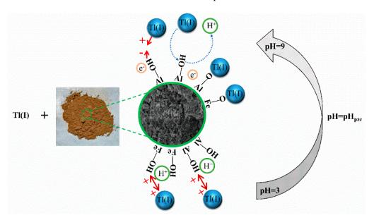
Figure 12. Mechanism diagram of Tl(I) adsorption by Al-WTR and Fe-WTR.
