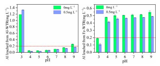
Figure 5. Effect of different pH conditions on the leaching of Al in Fe-WTR and Al-WTR.
