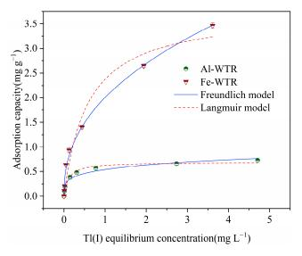
Figure 2. Isothermal adsorption model of Fe-WTR and Al-WTR for Tl(I).
