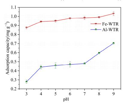
Figure 3. Effect of Fe-WTR and Al-WTR on Tl(I) adsorption under different pH conditions.
