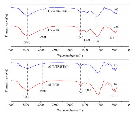
Figure 8. FTIR spectra of Fe-WTR and Al-WTR before and after adsorption.
