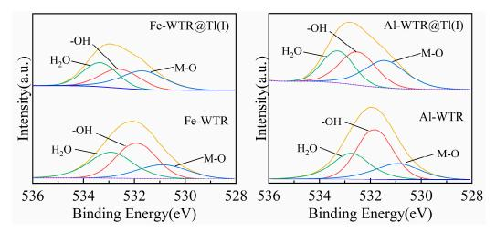
Figure 11. O 1 s spectra of Al-WTR and Fe-WTR before and after adsorption.
