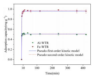
**Figure 1.** Kinetics of adsorption of Tl(I) by Fe-WTR and Al-WTR.
