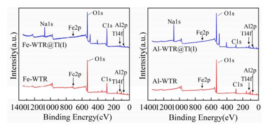
Figure 9. XPS spectra of Al-WTR and Fe-WTR before and after adsorption.
