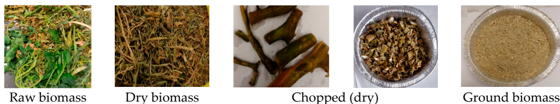
Figure 1. Biomass preparation steps for HTC process.
