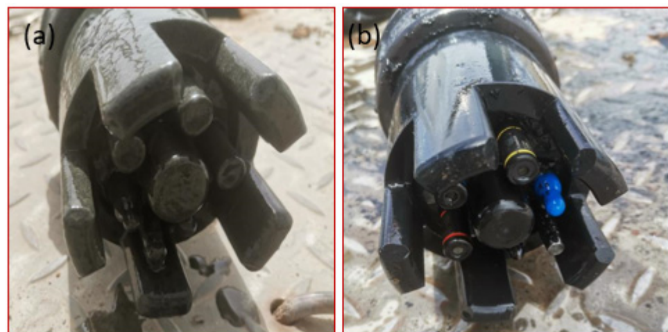
Figure 1. The integrated ammonium and nitrate sensors. (a) Being used for raw wastewater monitoring in influent channels for 24 h without cleaning; (b) after cleaning.
