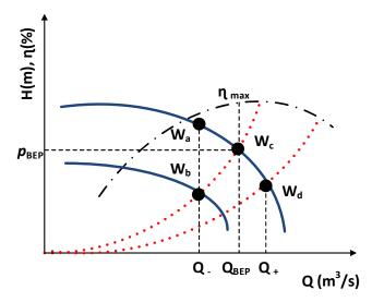
Figure 2. *H*-*Q* plane of pumping unit's operation.
