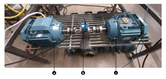
Figure 7. Experimental setup. (a) IM, (b) torque sensor, (c) SynRM.
