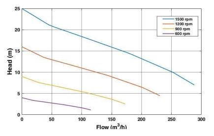
Figure 5. Family of performance curves of Grundfos SE 1.85.150 for a set of various rotational speeds.
