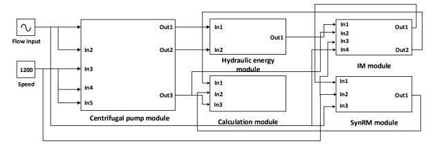
Figure 3. Structure of Simulink model.
