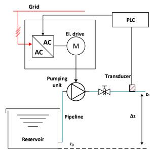
**Figure 1.** The general structure of the pumping system. Pipeline is presented by blue color and grid connection by red line.
