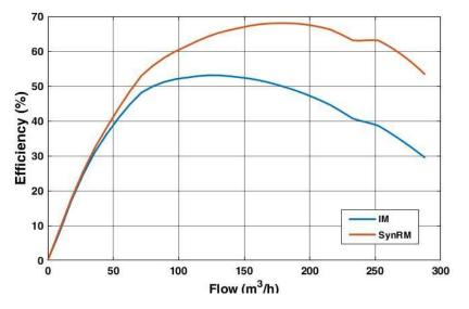
Figure 10. Comparison of IM and SynRM motor drives in pumping application.
