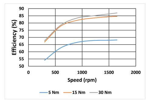
Figure 8. Family of efficiency curves for IM.
