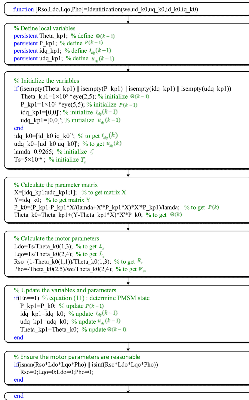
Figure 5. The function to realize RLS parameter identification.
