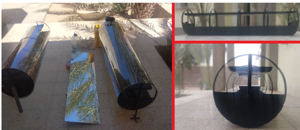
Figure 2. Real prototype of the novel solar still design.
