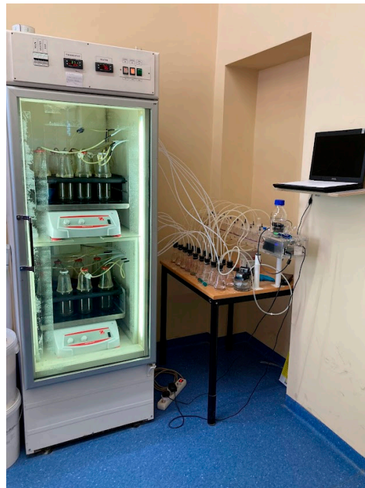
Figure 3. Batch BMP test system with an incubator capable of maintaining temperatures between 25 and 60 °C, orbital shaker (Ohaus-HEAVY DUTY ORBITAL SHAKERS) that provides a rotating orbital of 2 cm and a maximum rotation speed of 500 RPM.
