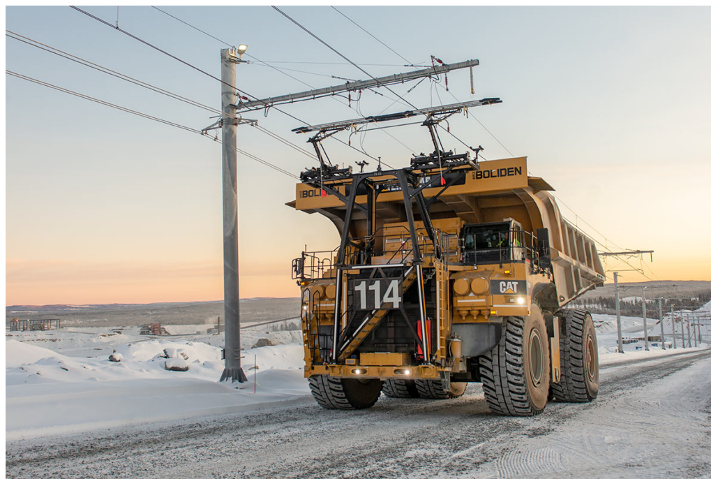
Figure 1. Haul truck connected to an overhead electric road system in the Aitik mine. (Picture: Mats Hillblom).
