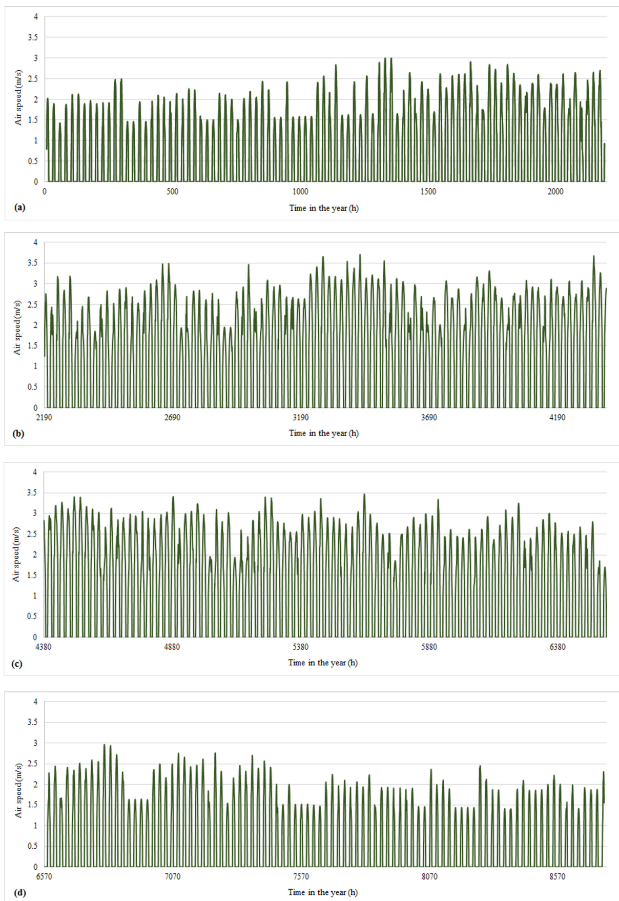
Figure 5. (a–d). Air speed in the solar chimney in each quarter of the year.
