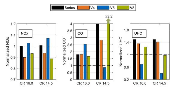
**Figure 15.** Comparison of different emissions for multiple compression ratios and geometries. Normalized with respect to CR 17.5.
