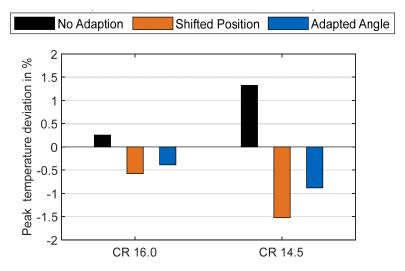
**Figure 11.** Comparison of peak mean in-cylinder temperature for injector position and spray-angle variation. Normalized with CR 17.5.
