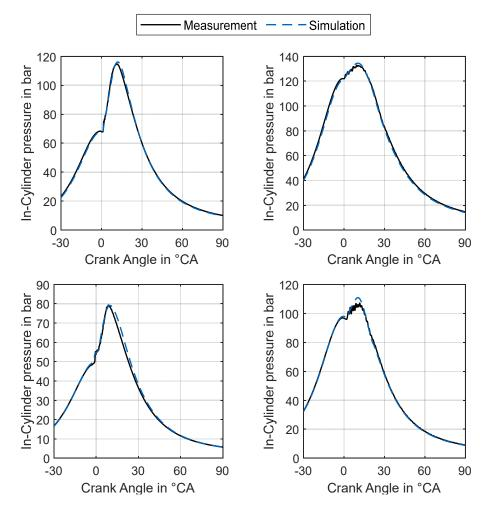
Figure 2. Pressure curve comparison CFD and measurement: (top left) 1200 rpm and 189 Nm; (top right) 2800 rpm and 189 Nm; (bottom left) 1200 rpm and 95 Nm; (bottom right) 2800 rpm and 95 Nm.
