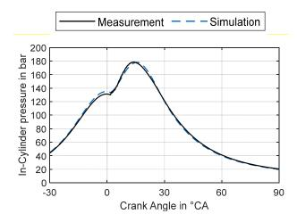
**Figure 3.** Pressure-curve comparison CFD and measurement: reference operating point at 1300 rpm and 401 Nm gross torque.
