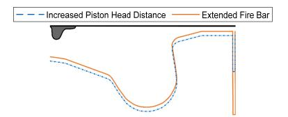
Figure 7. Piston-position comparison for compression-ratio variation.
