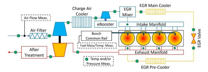
Figure 1. Schematic layout of the engine test bench.
