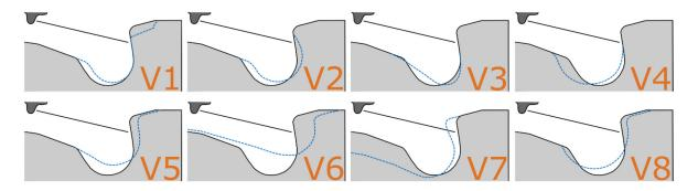
Figure 4. Eight new piston-bowl profiles compared to series geometry.
