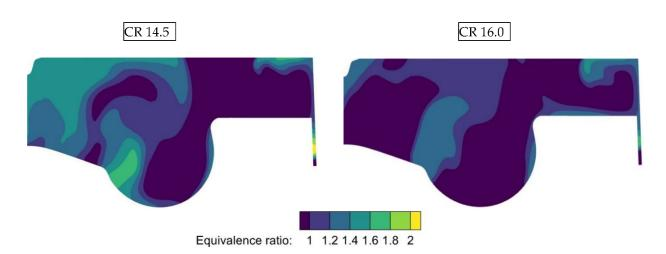
**Figure 16.** Piston bowl V8 for two compression ratios: equivalence ratio in sectional plane at 16 °CA. (left) CR 14.5; (right) CR 16.0.
