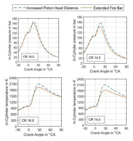
Figure 8. Compression-ratio-variation results. (top) Pressure curve; (bottom) temperature curve.
