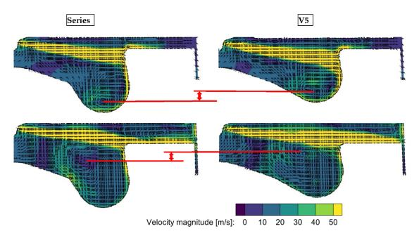
**Figure 5.** Lateral-vortex system during injection for series and V5: velocity including vectors in sectional plane. (**top**) 10 °CA after SOI; (**bottom**) 18 °CA after SOI.
