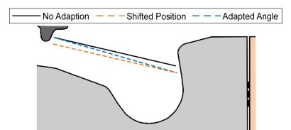
Figure 10. Spray directions for injector position and spray-angle variation at CR 14.5.
