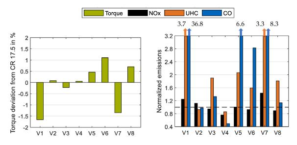
**Figure 6.** Comparison of torque and emissions for geometry variation. (**left**) Torque as deviation from series geometry; (**right**) specific emissions normalized with respect to series geometry.
