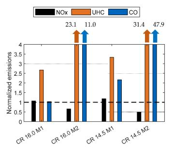
Figure 9. Comparison of different emissions for compression-ratio-reduction methods. (M1) Headpiston distance increase; (M2) fire-bar length increase. Normalized with respect to CR 17.5.
