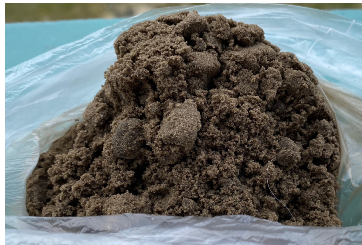
Figure 3. Sand obtained during well flushing in the workover process.
