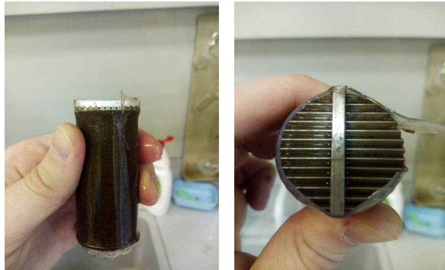
Figure 6. Bulk reservoir model with the preinstalled screen coupon (wire-wrapped screen (WWS) 200 \mu\text{m} ).
