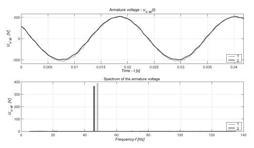
**Figure 8.** Phase-to-phase voltage  $U_{V-W}(t)$ : fault no. 3 to the governor speed controller. Load rate 100%  $P_n$ : 1, rated signal; 2, signal during the breakdown.
