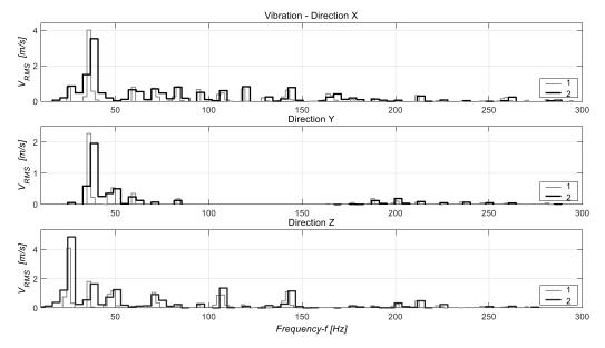
**Figure 9.** The fault at point 4 where the foundation frame is mounted to the ground—spectrum of the effective vibration velocity value: 1—rated signal; 2—signal during the breakdown.
