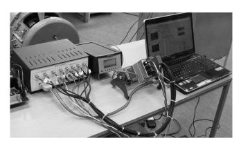
Figure 5. Modular computer subsystem used for measuring diagnostic parameters.
