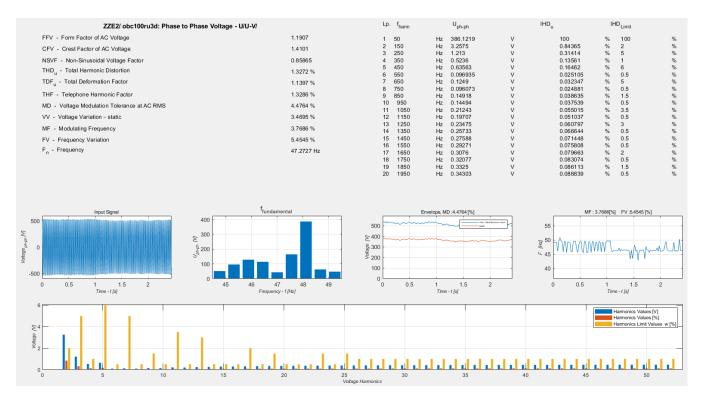
**Figure 6.** The MATLAB user interface of the ELPAR application: a set of analyses for synchronous generator armature voltages.
