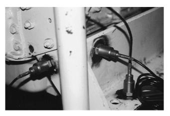
**Figure 4.** A view of the mounting point of the accelerometers on the foundation frame used for measuring vibrations in three directions.
