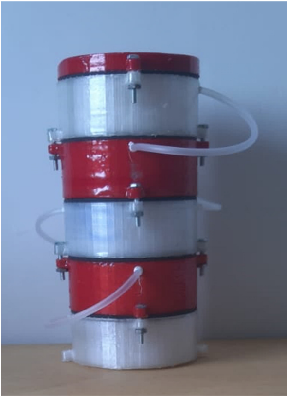
Figure 7. Reaction cells of the Cascade System for Biomineralization in Cement.
