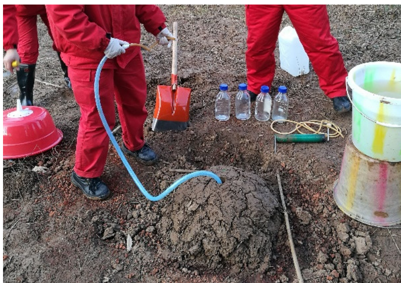
Figure 2. The method used to collect the leaking gas.
