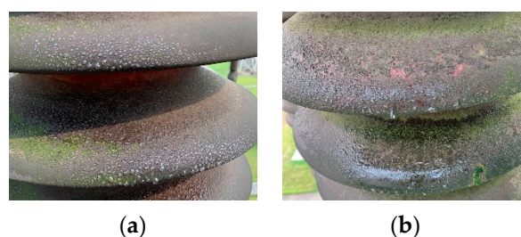
Figure 8. The hydrophobicity test results of the RTV post insulator. (a) Algae-free RTV surface. (b) Algal RTV surface.
