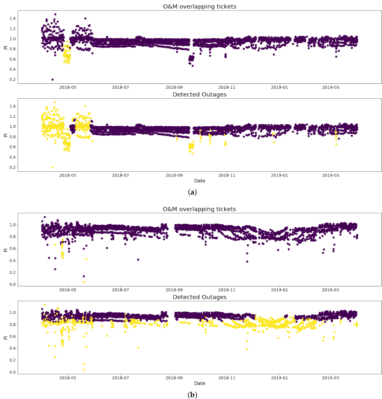
Figure 7. Visuals of two site-level data (a,b) show that more failures (points in yellow) are detected by PV-HMMs (“Detected Outages”) than captured in the maintenance tickets (“O&M overlapping tickets”). The purple points represent samples which have no detected outage.
