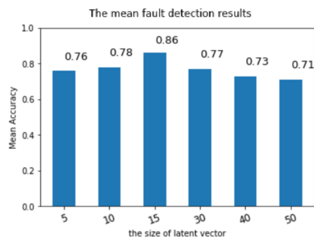
Figure 7. The mean fault detection results w.r.t. varying values of the latent vector size.
