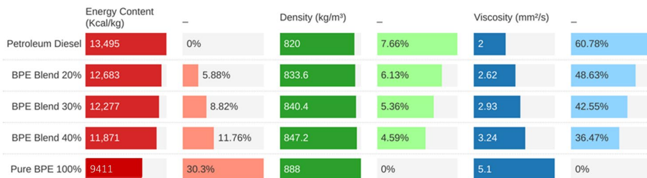
Figure 3. The main properties of the biodiesel blends gradually change with increasing biodiesel content in the mixture.
