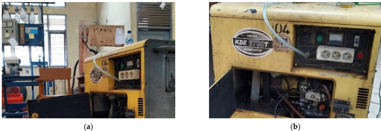
Figure 4. Experimental test apparatus: (a) KDE 6700T power generator and test instruments (b) modified external fuel line system bypassing default fuel tank.
