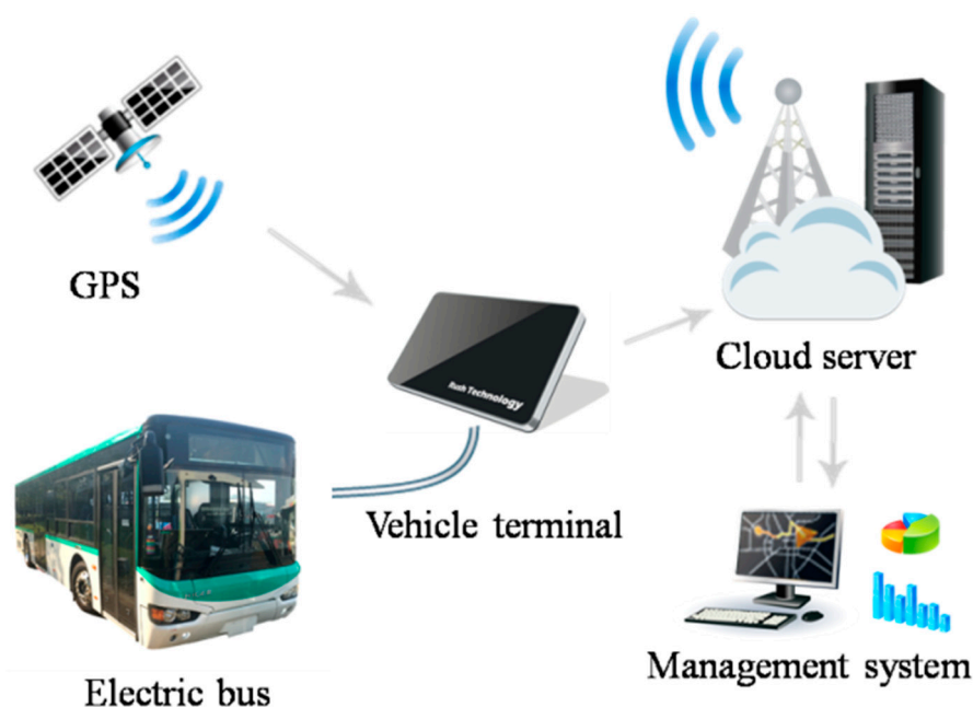
Figure 16. A test system for key early fault warning method of electric buses from Higer Bus Company Limited.
