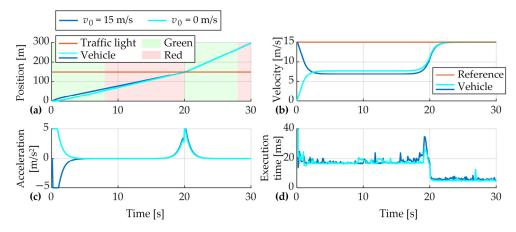
**Figure 8.** Comparative responses position (**a**), velocity (**b**), acceleration (**c**) and execution time (**d**) of linear MPC systems for initial vehicle velocities  $v_0 = 0$  and  $v_0 = v_R = 15$  m/s.
