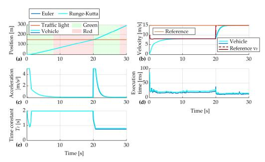
**Figure 11.** NMPC system responses for different time-discretization methods applied. Subfigures show position (a), velocity (b), acceleration (c), execution time (d) and time constant control input (e).
