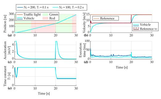
**Figure 12.** NMPC system responses for different sampling time values. Subfigures show position (a), velocity (b), acceleration (c), execution time (d) and time constant control input (e).
