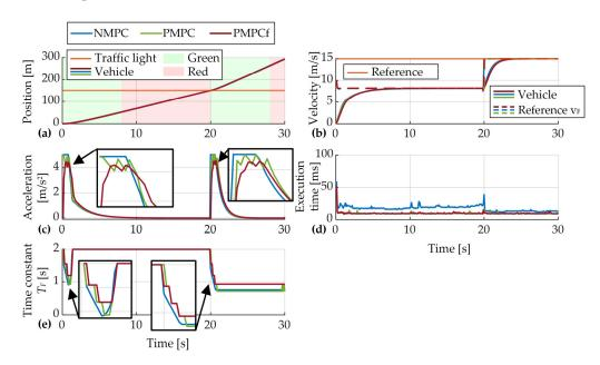
**Figure 14.** Comparative responses of position (**a**), velocity (**b**), acceleration (**c**), execution time (**d**) and time constant input (**e**) of NMPC, PMPC, and PMPCf systems.
