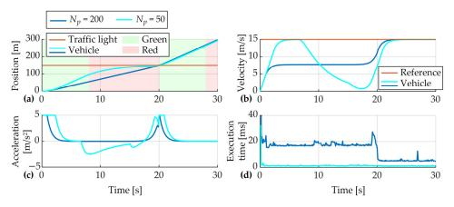
**Figure 7.** Comparative responses position (**a**), velocity (**b**), acceleration (**c**) and execution time (**d**) of linear MPC systems for prediction horizon lengths  $N_p = 200$  and  $N_p = 15$ .
