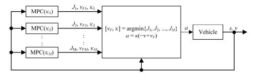
Figure 5. Block diagram of parallel MPC.
