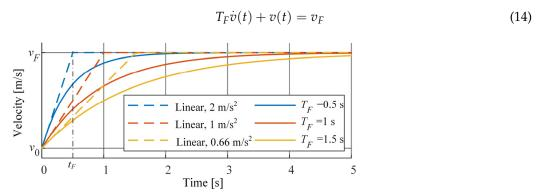
Figure 4. Illustration of nonlinear MPC velocity trajectory.
