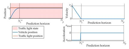
**Figure A1.** Illustration of the shortest control horizon case for feasible linear MPC with reduced control horizon ( $N_c \ll N_p$ ).
