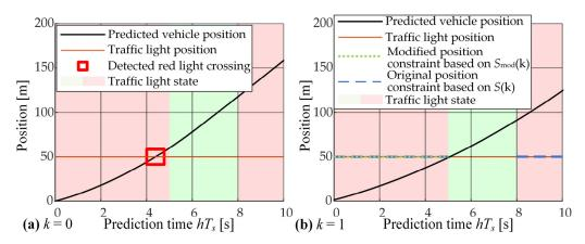
Figure 2. Illustration of construction of time-dependent only traffic light position constraint in current time step (b) based on vehicle position trajectory predicted in previous step (a).
