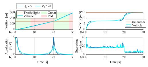
**Figure 10.** Illustration of influence of acceleration weighting coefficient  $q_a$  on position (**a**), velocity (**b**), acceleration (**c**) and execution time (**d**).
