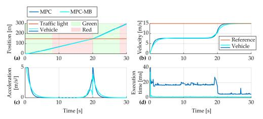
**Figure 9.** Comparative responses position (**a**), velocity (**b**), acceleration (**c**) and execution time (**d**) of nominal and move-blocking (MB) linear MPC systems.
