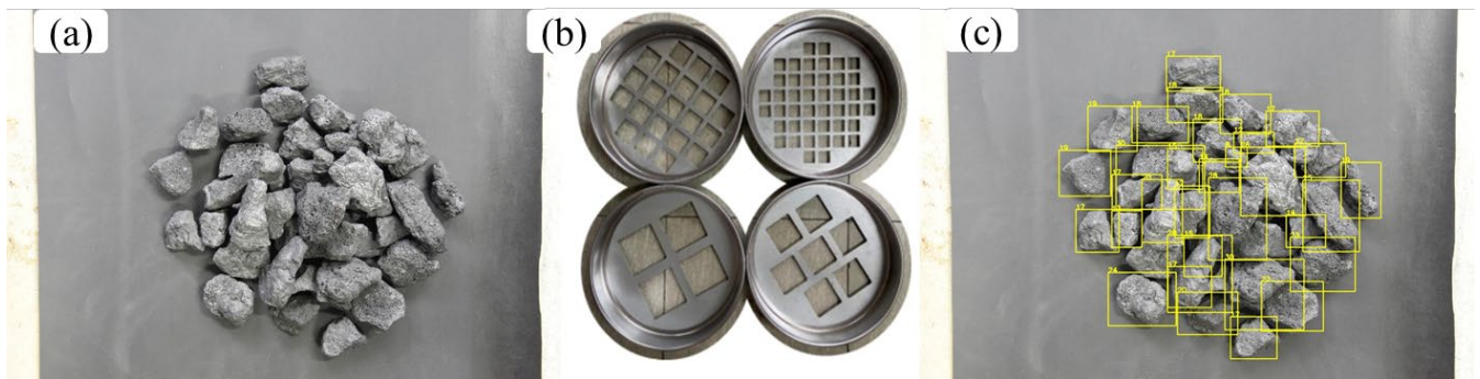
Figure 13. Example of a coke image. (a) Coke image; (b) Square hole sieves; (c) Detection sizes of coke particles.
