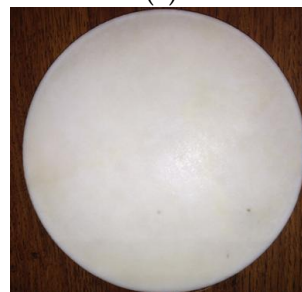
Figure 2. (a) plenum design (b) Distributor for 0.14 m and 0.44 m fluidized bds made of a porous Polyethylene sheet with a pore Size of 15–40 \mu\text{m} .
