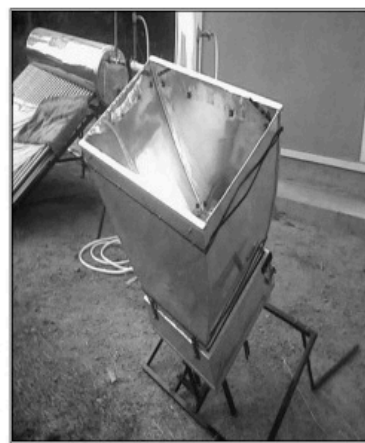
Photograph of box cooker implemented with CPC-45 collector
