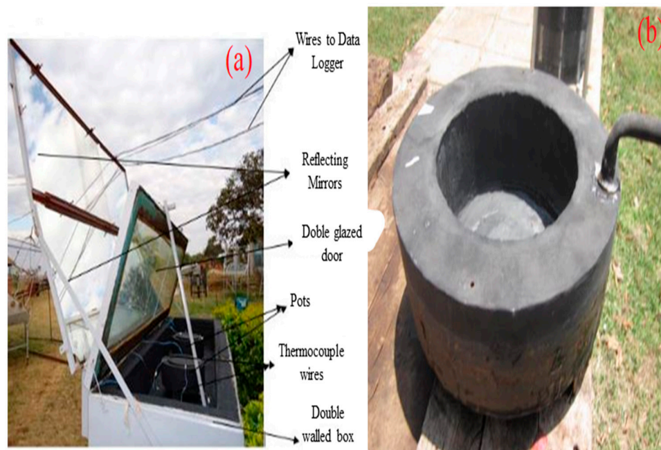
Figure 22. Solar cooker set with PCM storage unit: (a) Experimental setup; (b) PCM storage unit. Reprinted/adapted with permission from Ref. [66], 2019, Jomo Kenyatta University of Agriculture and Technology.
