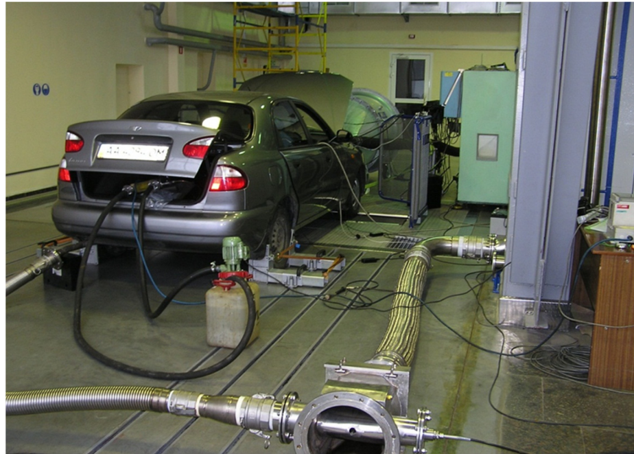
Figure 3. The 2007 Daewoo Lanos during bench tests.
