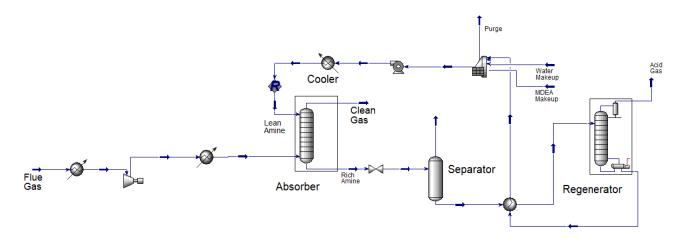
Figure 13. Process flow diagram of the MDEA CO<sub>2</sub> capture process.
