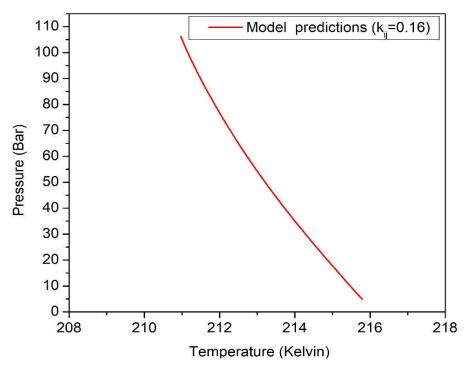
Figure 6. Model predictions for SLVE locus of the binary system O<sub>2</sub>-CO<sub>2</sub>.
