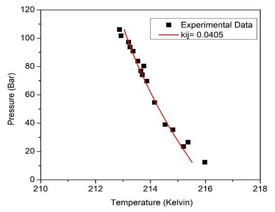
**Figure 4.** Comparison of model correlation of the SLVE PT locus (line) with the optimum kij value to the corresponding experimental data (symbols) for the binary system N<sub>2</sub>-CO<sub>2</sub> [22].
