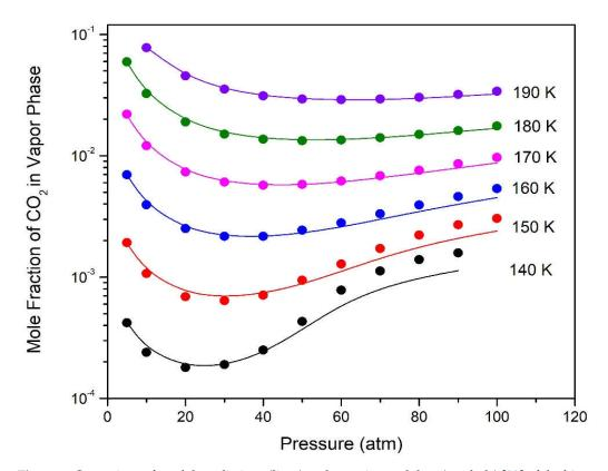
**Figure 5.** Omparison of model predictions (lines) and experimental data (symbols) [22] of the binary system N<sub>2</sub>-CO<sub>2</sub> for the effect of temperature and pressure on composition of vapor phase in the SVE region.
