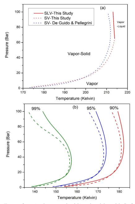
**Figure 8.** Comparison between results of this study and those of the De Guido and Pellegrini study [24] for the CO2 recoveries of (**a**) 0% (frost line) and (**b**) 90%, 95%, and 99% recovery. Solid and dashed lines represent this study and the study of De Guido and Pellegrini, respectively [31].
