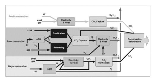
**Figure 1.** The three main approaches for CO<sub>2</sub> capture [5].
