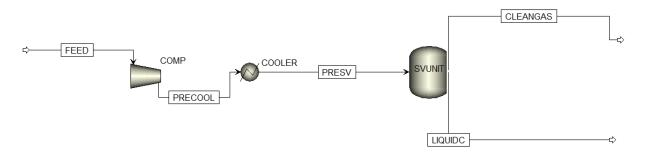
Figure 9. Process flow diagram of the SV CO<sub>2</sub> capture process.
