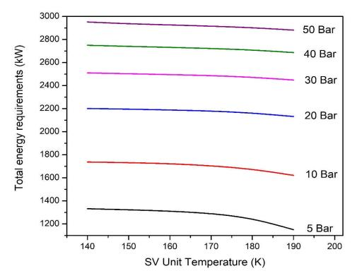
**Figure 12.** Combined impact of compressor discharge pressure and SV unit operating temperature on the total energy rate consumption of the SV CO<sub>2</sub> capture process.
