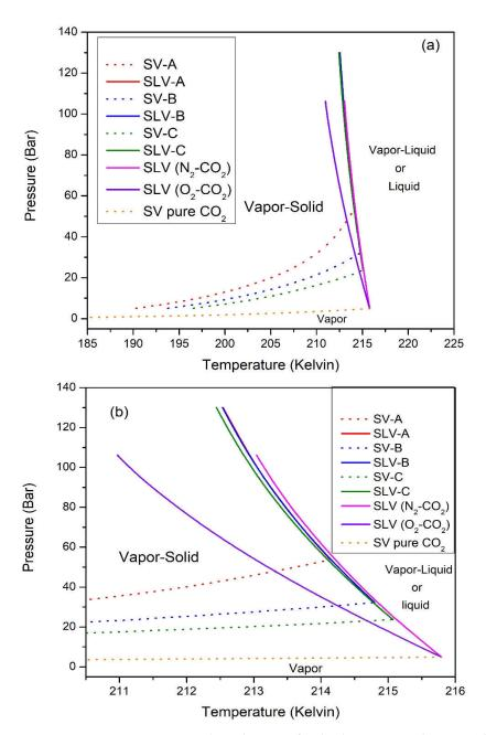
**Figure 7.** Pressure–temperature phase diagrams for the three cases and compared to SLV locus lines for the binary systems;  $N_2$ -CO<sub>2</sub> and O<sub>2</sub>-CO<sub>2</sub>: (**a**) over the full range of temperatures, and (**b**) zoomed into the temperature range 210.5–216 K.
