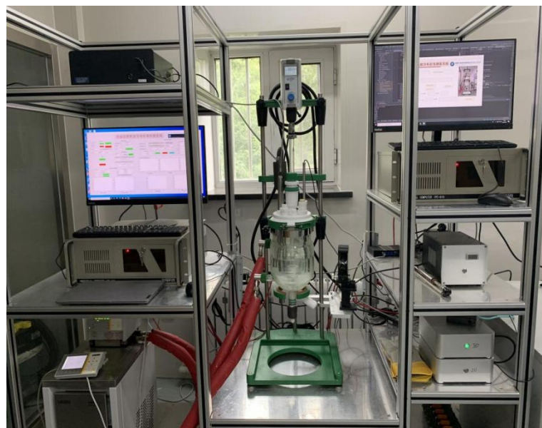
Figure 6. Experimental equipment for batch cooling crystallization processes.
