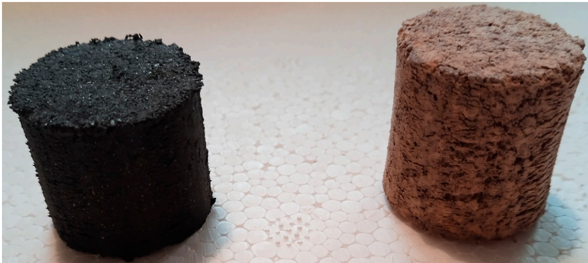
Figure 2. Starting (left) and roasted at 1150 °C for 65 min (right) compacted samples.
