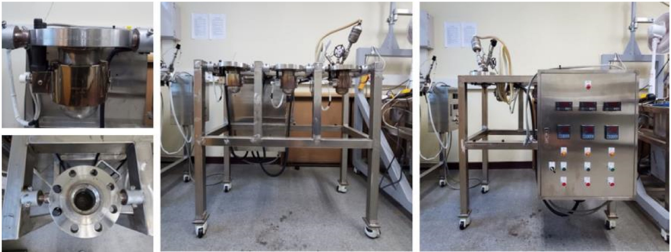
Figure 1. Laboratory-scale hydrothermal carbonization reactor (0.2 L).
