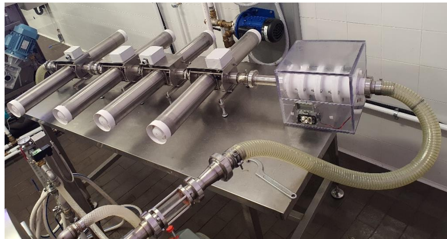
Figure 3. Continuous-flow extraction under combined US (C2FUT Srl) and PEF (Energy Pulse Systems), DSTF—University of Turin.
