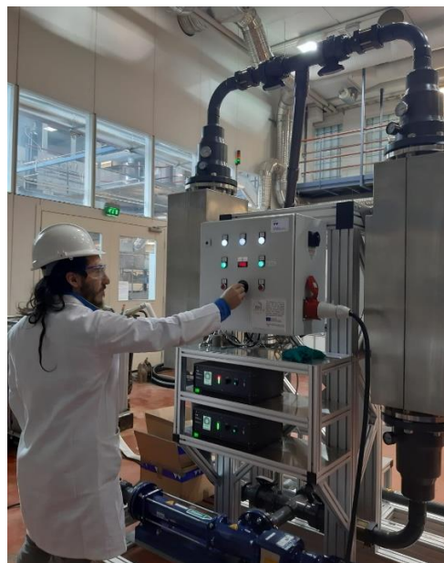
Figure 1. Semi-industrial US flow reactor (Weber Ultrasonics AG) for biomass pretreatment.
