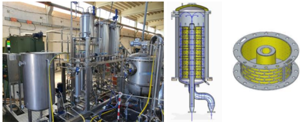
Figure 7. Pressure-resistant reactors for SWE (C2FUT Srl.). Left: plant photo; right: reactor tank and loading vessel scheme, DSTF—University of Turin.
