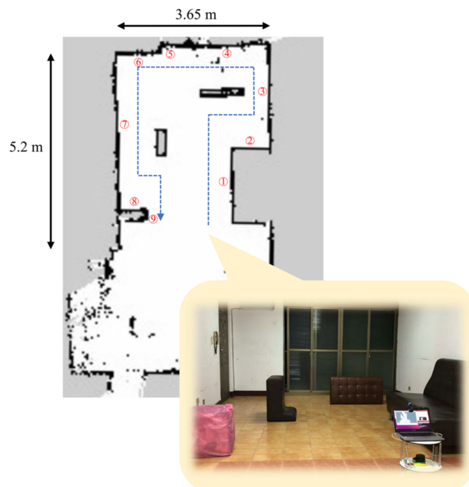
Figure 32. Mapping results of first environment, number 1–9 mean the length of each side.
