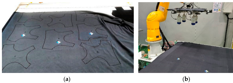
Figure 13. Automatic cutting process: (a) preparation for cutting; (b) transfer of cut fabrics for robot gripping.
