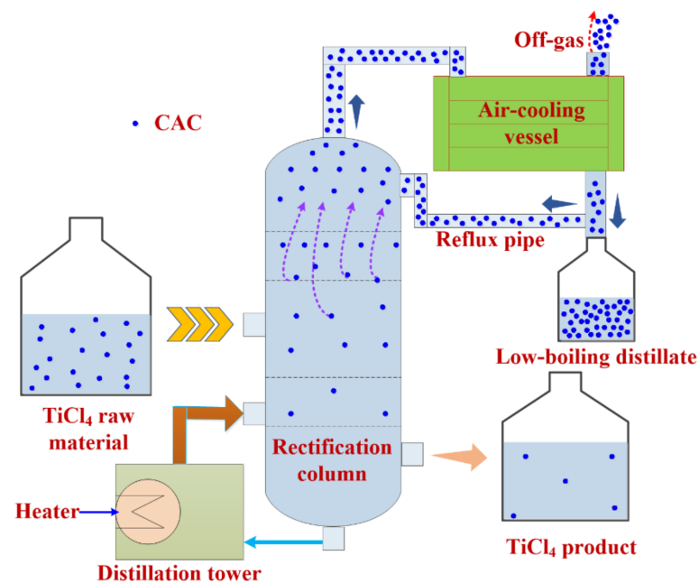
Figure 2. Schematic illustration of the TiCl 4 rectification.
