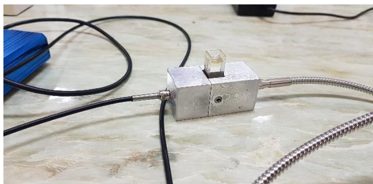
Figure 2. Measurement of VIS/near infrared (NIR) spectra of pesticide in passing mode.
