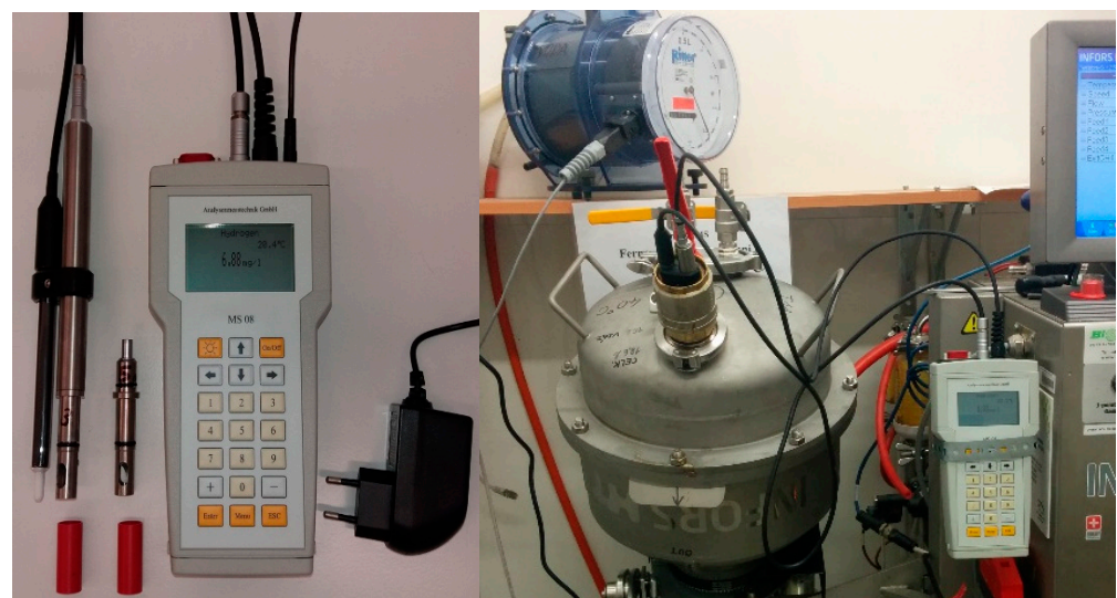
Figure 2. Amperometric microsensor and its location in the reactor.
