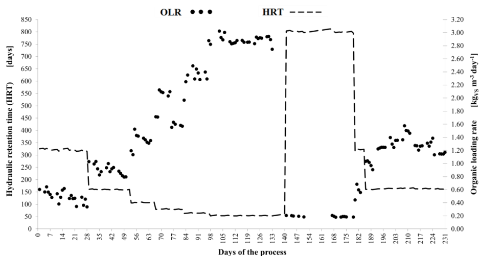
Figure 3. Relation between organic loading and retention time.
