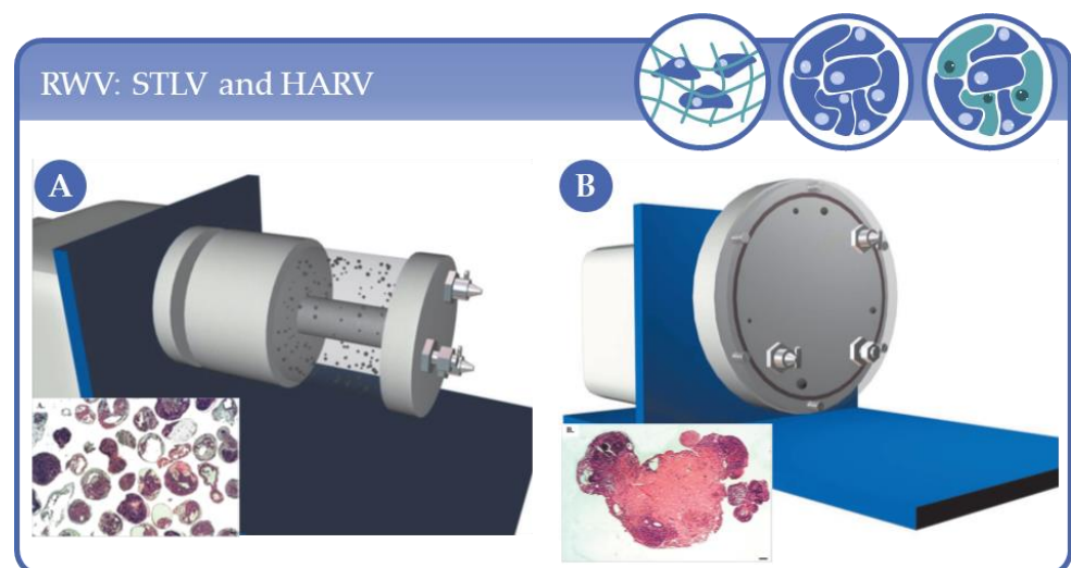
Figure 8. Diagram of two types of rotating wall vessel (RWV) bioreactors. (A) Slow turning lateral vessel (STLV) for formation of smaller cell aggregates (in this case small human embryoid bodies). (B) Usage of a high aspect rotating vessel (HARV) bioreactor leads to agglomeration of big cellular clumps. Reprinted from [45] with permission of John Wiley and Sons.
