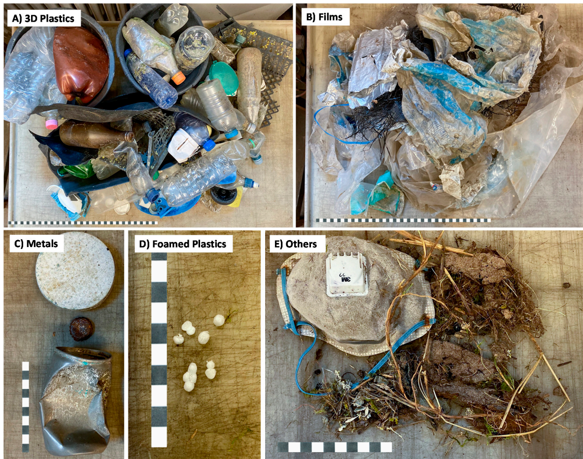
Figure 4. ML fractions Norderney: (A) 3D Plastics; (B) Films; (C) Metals; (D) Foamed Plastics and (E) Others. The scale amounts to 1 cm per section (Picture: Jacqueline Plaster, Johann Hee).
