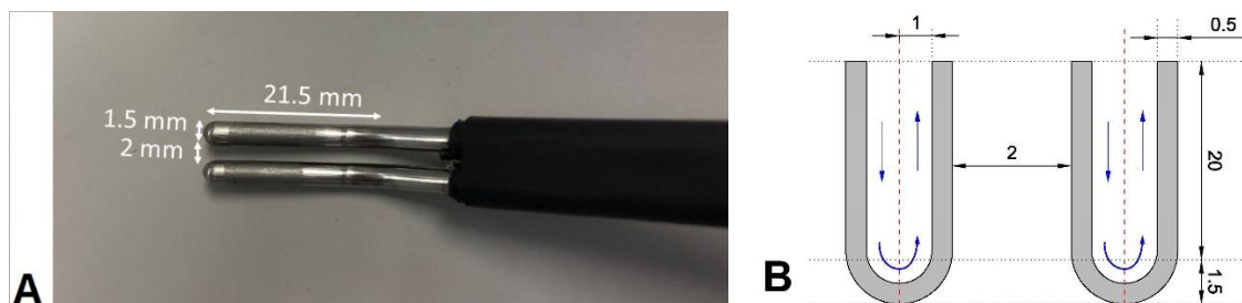
Figure 2. (A) Bipolar RF applicator used to consider the geometry of the computational model. (B) Scheme of the electrodes' tips included in the bipolar RF applicator of the left picture (in mm, out of scale).
