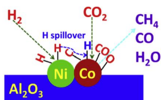
Figure 6. Synergistic effect proposed for x\text{Co}-y\text{Ni}-\text{Al}_2\text{O}_3 catalysts [80]. Reproduced with permission from Xu et al., International Journal of Hydrogen Energy ; published by Elsevier, 2018.
