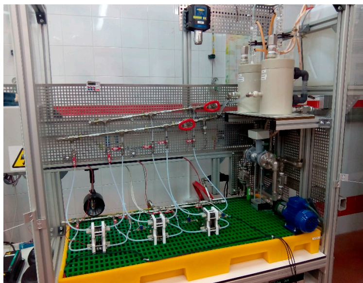
Figure 5. Alkaline water electrolysis cell test bench of the Centro Nacional del Hidrógeno .
