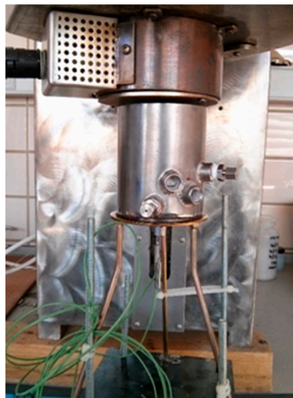
Figure 4. Coupling of the melting furnace outlet and the cooling device.
