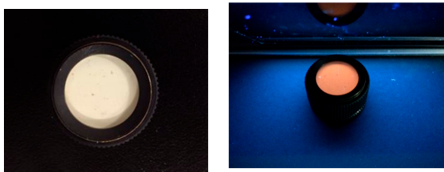
Figure 2. Image of the L-Cys/Au(I) complex without (left) and with (right) black light irradiation (wavelength 365 nm).
