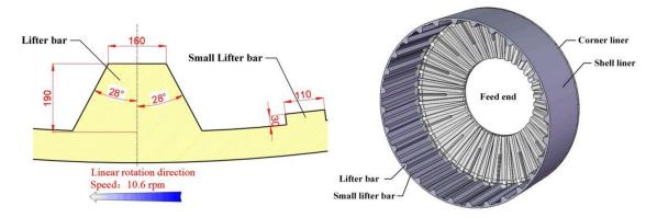
Figure 4. Cylinder model for simulation.
