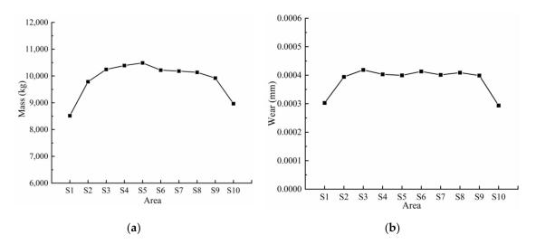
**Figure 6.** (a) The total mass of particles in each area in the simulation at 40 s. (b) The average cumulative wear of each area in the simulation at 40 s.
