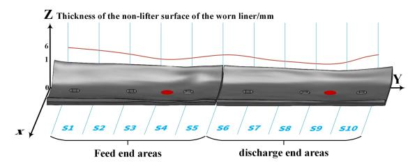
Figure 3. Schematic diagram of the liner area division and thickness of the bottom surface.
