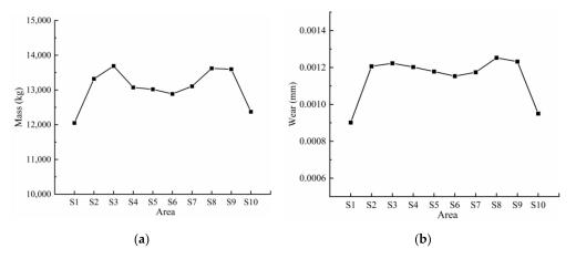
**Figure 5.** (a) The total mass of particles in each area in the simulation at 60 s. (b) The average cumulative wear of each area in the simulation at 60 s.
