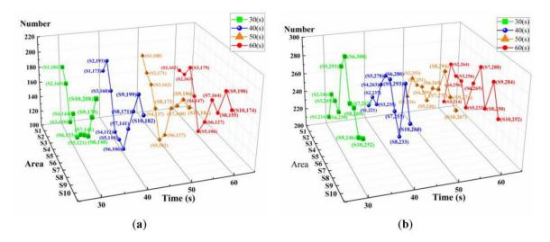
**Figure 8.** (a) The number of 200 mm rocks distributed in each area at each time point. (b) The number of 110 mm steel balls distributed in each area at each time point.
