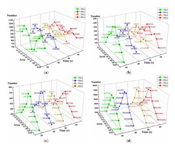
**Figure 9.** (a) The number of 180 mm rocks distributed in each area at each time point. (b) The number of 90 mm steel balls distributed in each area at each time point. (c) The number of 70 mm steel balls distributed in each area at each time point. (d) The number of 60 mm rocks distributed in each area at each time point.
