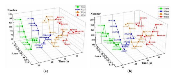
**Figure 7.** (a) The number of 150 mm steel balls distributed in each area at each time point. (b) The number of 130 mm steel balls distributed in each area at each time point.
