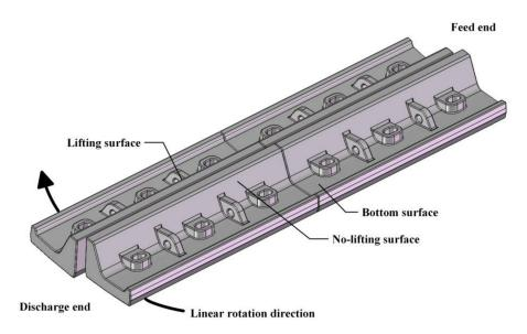
Figure 1. Arrangement model of the cylinder liner.
