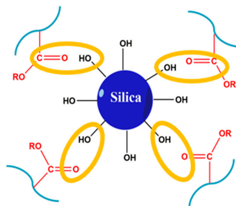
Figure 6. Schematic diagram of the hydrogen bonding interaction between itaconate elastomer and silica.
