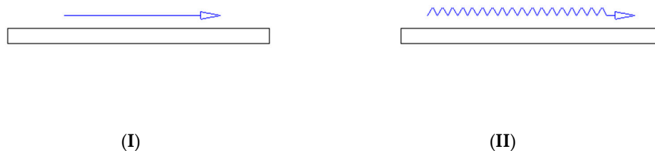
Figure 4. The comparison of product movement between a shaken conveyor and a vibrating conveyor. (I)—shake conveyor—product movement. (II)—vibrating conveyor—product movement.
