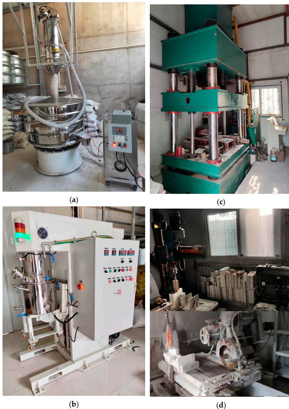
Figure 4. Equipment for making synthetic sandstone: (a) mechanical sieve with an automatic feeder; (b) 20 L mechanical mixer; (c) 500-ton hydraulic press; (d) coring drill/table saw.
